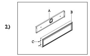
Step.2: Install lamp body (B) to back plate using two screws (C) on the sides.
